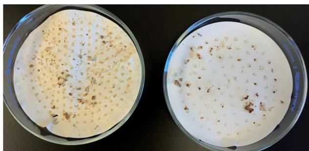
Fig. 7 Extracts collected in the membrane filter after continuous (left) vs. sequential WPO (right).
