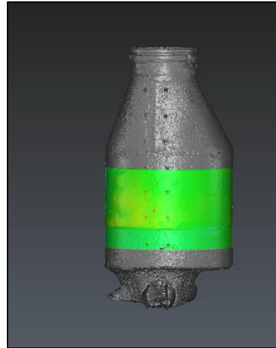
Manhole Virtual Model (MVM™) (Diameter, Elevations, Material)
